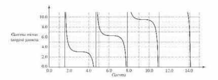
The graph above is a plot of  $f(\gamma) = \gamma - \tan \gamma$ . So when it equals zero, one has an intensity maximum. Getting estimates from the graph, and then using trial and error to narrow in on the value, we find that the three smallest  $\gamma$ -values are  $\gamma = 4.49$  rad 7.73 rad, and 10.9 rad.
